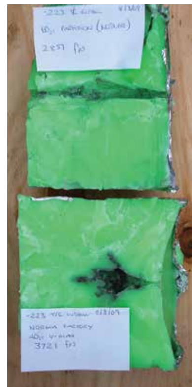
Above: This shows the difference between a heavy bullet passing through (top) and a high velocity light one expanding with no exit (bottom).
